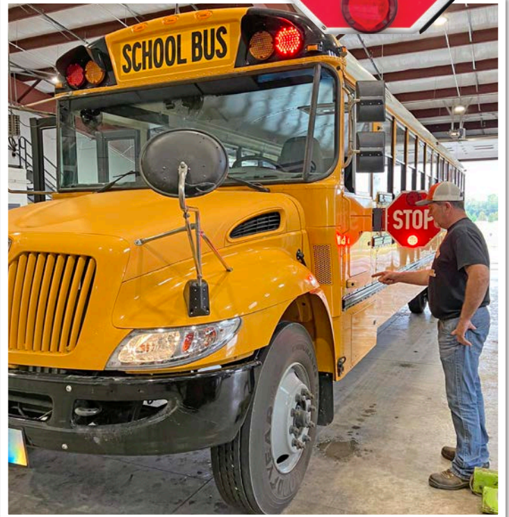
Transportation Director Todd Conant points to the small video camera that activates automatically if a vehicle passes while the bus's flashing red light arm is extended. All Mount Vernon City Schools buses are equipped with the cameras.
